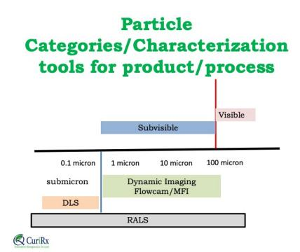
Right Angle Light Scattering (RALS) represents macroscopic changes in an otherwise soluble molecule transferring to aggregation. When a molecule unfolds and aggregates, it scatters light.
